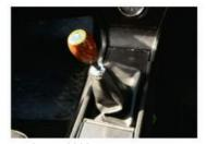
The Corsair 2000E **transmission** was standard, with the close-ratio Lotus 'box optional for competition. Test for worn synchros and jumping out of top gear
