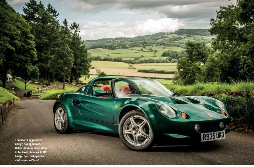
Lotus practice but which, after the excessively complicated make-up of the M100 Elan, was pared back to the minimum. With just eight panels, it employed half the number used in the M100, thus streamlining the production process and improving quality. Penned in-house by Thomson and selected in preference to 11 other proposals from external design consultancies, the slinky skin was stretched tautly over the four corners like a pair of Lycra shorts.
