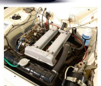
The Cortina II Lotus Twin Cam was originally fitted with a large air-cleaner box atop the cylinder head to reduce induction noise. Worn **engines** become smoky and are reluctant to start – Weber carburettors don't go out of tune quickly, so be highly suspicious of vendors who blame the carbs for a smoky engine...
