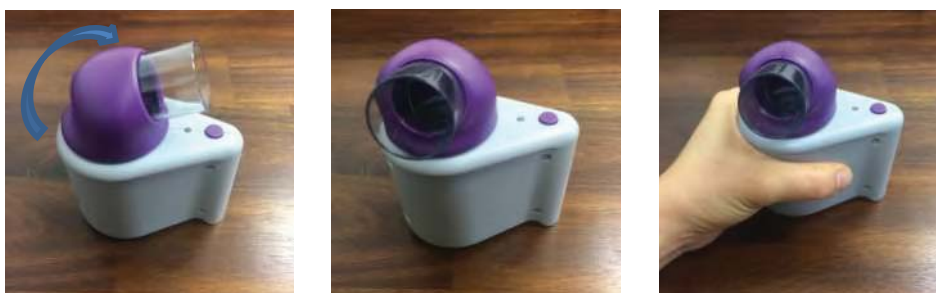
Figure 2 Insert transducer for left hand use
