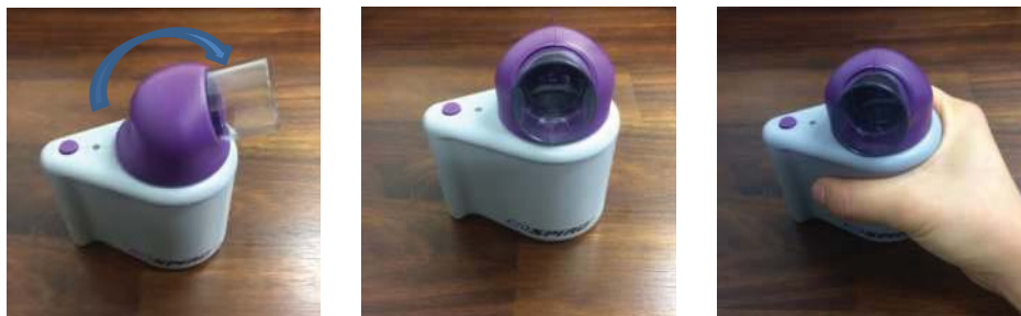
Figure 1 Insert transducer for right hand use
