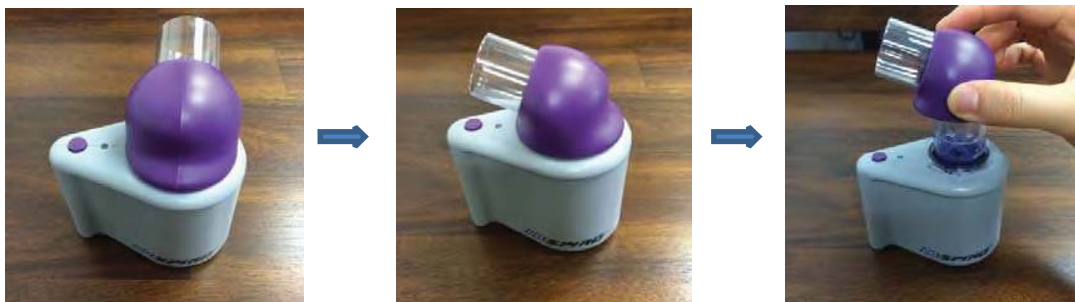
Figure 6 removal of transducer if you use GoSpiro with left hand
