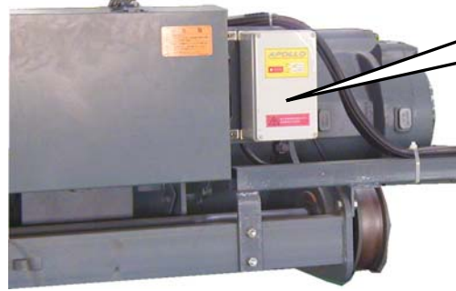
( fig. 1 ) ( example for fix / install receiver )
