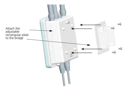
**4** Attach the bridge with bracket to the plate already fixed to the pole.
