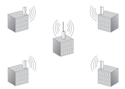
The following figure shows a point-to-multipoint "in-line" configuration with one bridge set to "Master" and using a directional panel antenna.
