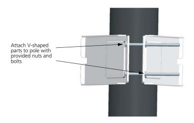
**2** Fit the edges of the V-shaped part into the slots in the rectangular plate, and tighten the nuts.
