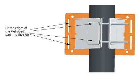
**3** Attach the adjustable rectangular plate to the bridge with supplied screws.
