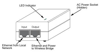
The wireless bridge does not have a power switch. It is powered on when its Ethernet port is connected to the power injector module, and the power injector module is connected to an AC power source. The power injector includes one LED indicator that turns on when AC power is applied.
