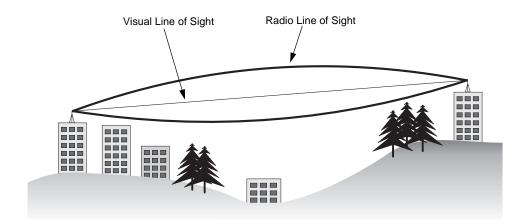
If there are obstacles in the radio path, there may still be a radio link but the quality and strength of the signal will be affected. Calculating the maximum clearance from objects on a path is important as it directly affects the decision on antenna placement and height. It is especially critical for long-distance links, where the radio signal could easily be lost.
