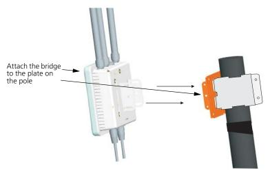
**5** Use the included nuts to secure the wireless bridge to the pole bracket. Note that the wireless bridge tilt angle may need to be adjusted during the antenna alignment process.
