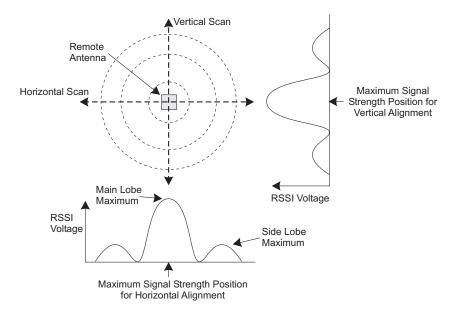
To align the antennas in the link, monitor the signal strength LEDs or the RSSI value in the management interface. Start with one antenna fixed and then perform the following procedure on the other antenna:
