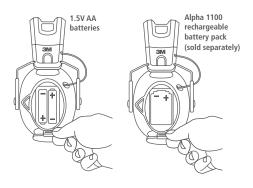
Install two 1.5V AA batteries or optional Alpha 1100 rechargeable battery pack as shown. Replace battery door top-end first.
