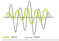
Clear Voice Tracking seeks voices in background/ environmental noise and reduces the noise to improve speech intelligibility. The user can select standard microphone filtering by turning off the Surround Sound Filtering in the setup menu. The default setting is Surround Sound Filtering ON.
