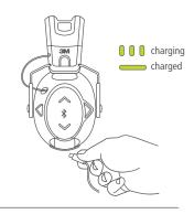
Insert the micro-USB connector cable into the micro-USB jack. Connect the other end of the cable to a USB power source to begin charging.
