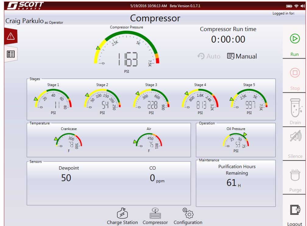
Figure 10 HMI Compressor Screen
