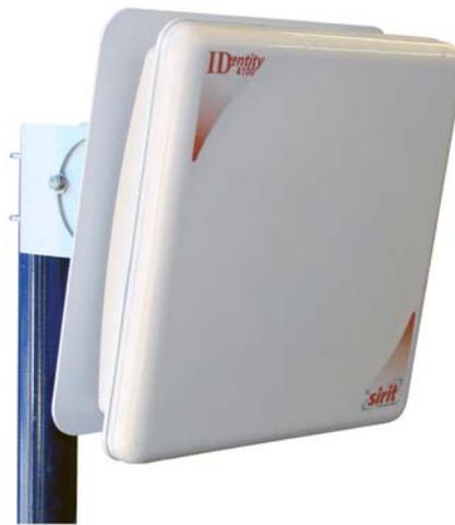
**Figure 1** IDentity 4100 UHF Reader with Universal Mount
