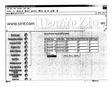
Active state can be set to active low or active high and the there are three options for output drive state. Open drain, Push pull, and none.
