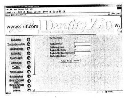
The duplicate filter will remove all subsequent instances of a particular tag after the initial read. This can greatly reduce the amount of data reported back to the user caused by a tag remaining in the read zone for a longer
