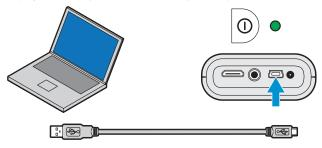
Important Note: To conserve power, the projector will stop projecting an image while connected to a computer USB port.
