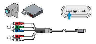
Important Note: There are two red connectors on the Component AV cable. One is for the right audio channel and the other is for the Pr component video signal. Be careful to connect the red audio to red audio and red video to red video. If these connectors are switched, the projected image will appear green and an abnormal noise will come from the right speaker.
