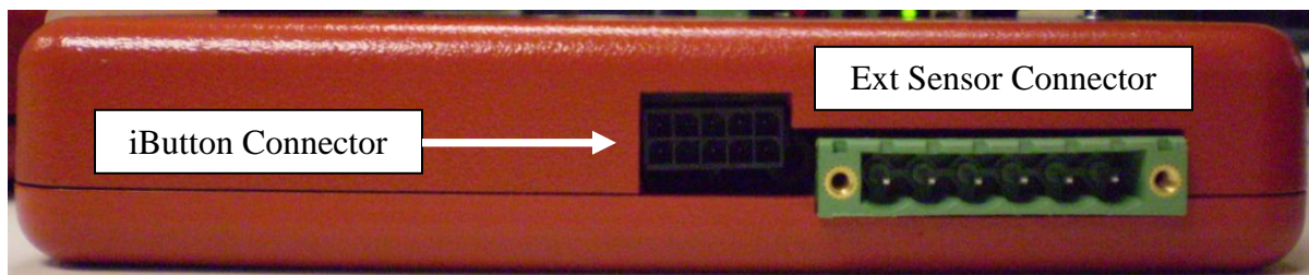
MCU side view with iButton/serial interface connector and ext sensor terminal block
