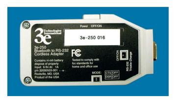
Once you have configured the dipswitches, connect the 3e-250 to the DB9 connector on the test instrument. If there is not enough space to directly connect to the DB9 connector, use a 9-pin straight cable with a male connector at one end and a female connector at the other. (This is not included in the install kit.)
