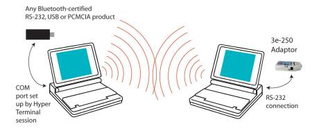
At this point, you have completed the communication setup between the 3e-250 Adapter and the other Bluetooth device.
