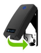
Secure the reader module to the backplate using the M3x100mm screw as supplied.
