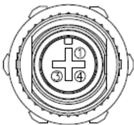
Pin Assignments Front View
