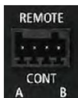
The inputs are logic inputs with 4700  $\Omega$  pullup to +3.3 VDC. They require a pull down to ground to activate the control. The ground potential is available on the connector (see 'Protection Switch Remote Control Connections' on page 367).
