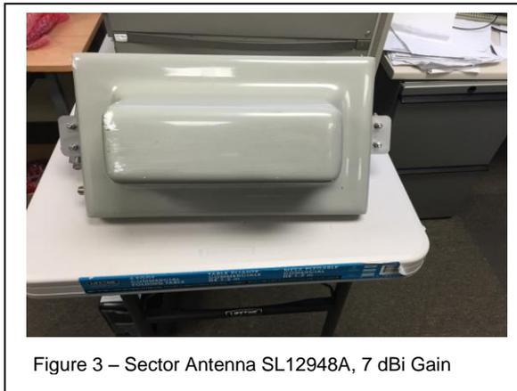
Figure 3 – Sector Antenna SL12948A, 7 dBi Gain
