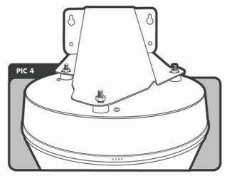
There are three elliptical holes in the wall-mount mechanics. Mount the Eye unit by pushing the screws on top of the unit through the wall-mount mechanics. From the top-side of the mechanics use the screws to attach the unit to the mechanics.
