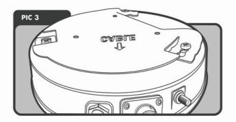
Insert the screws into the holes in the roof mounting plate. Turn the unit and feel it snatching into the plate. The unit should not be moving in a loose manner but it moves only few millimeters when properly mounted.
