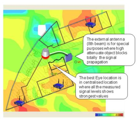
The external antenna is useful in the environment where shafts or thick walls are attenuating radio too much.
