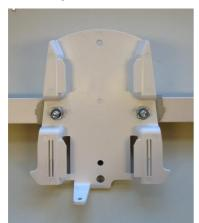
Slide the Indoor Eye onto the bracket and secure it with the #6 Phillips head screw.
