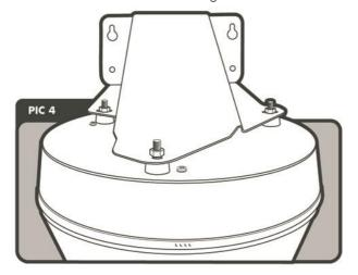
There are three elliptical holes in the wall-mount mechanics. Mount the Eye unit by pushing the screws on top of the unit through the wall-mount mechanics. From the top-side of the mechanics use the nuts to attach the unit to the mechanics.
