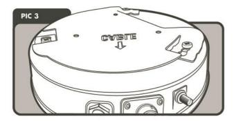
Mount the Eye unit on the ceiling mounting plate by inserting the screw tops into the plate holes. Make sure that the marking 'CABLE' is pointed towards connectors. Turn the unit and feel it snatching into the plate.
