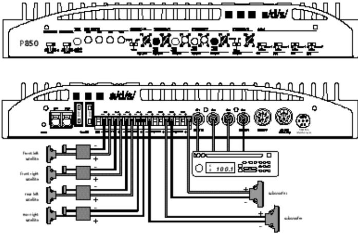
System 2 – The P850 is used in 8-channel mode. Channels 1/2 are high-passed for front tweeters. Channels 3/4 are band-passed for front midrange. Channels 5/6 are high-passed for rear speakers, and channels 7/8 are low-passed for subwoofers. Although shown as a 4-channel input, the source unit can be either 2- or 4-channel.
