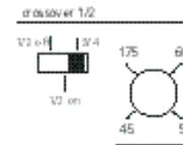
Note: When the switch is in the right position, the output level is controlled by the ch 3/4 level control.
