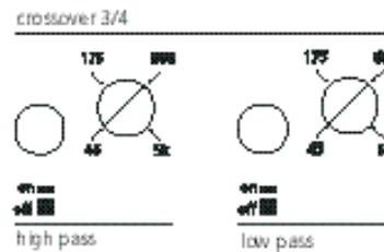
cover control 3/4 – The crossover section dedicated for channels 3 & 4 are activated by depressing the switch next to each frequency adjustment control. Both high-pass and low-pass crossovers are infinitely adjustable from 45Hz to 5,000Hz. The high-pass and low-pass sections may be used individually or together to create a band-
