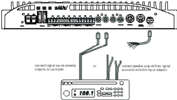
High-level MiniDin input connections:
