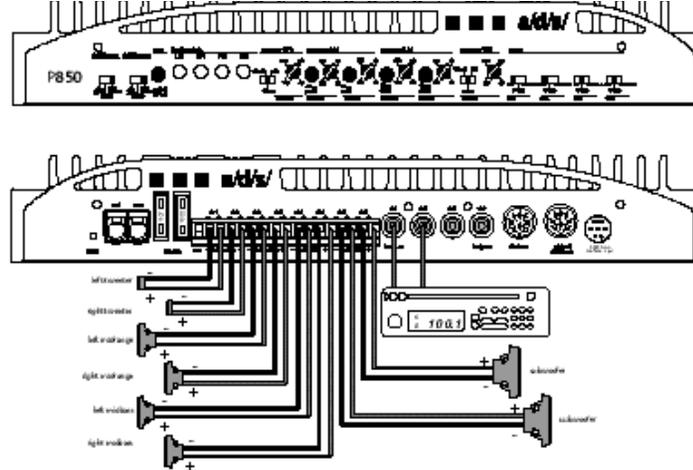
System 4 – The P850 is used in bridged 4-channel mode. Channels 1/2 and 3/4 are high-passed bridged-mono for front speakers. Channels 5/6 and 7/8 are low-passed summed bridged for subwoofers. Front speaker level control is adjusted by the ch3/4 level control. Subwoofer level is controlled by the ch5/6 level control. the P840.2 is configured for 2-channel input.
