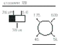
When the switch is in the left position, the crossover section of the amplifier is bypassed. Channel 7 & 8 output is full range.
