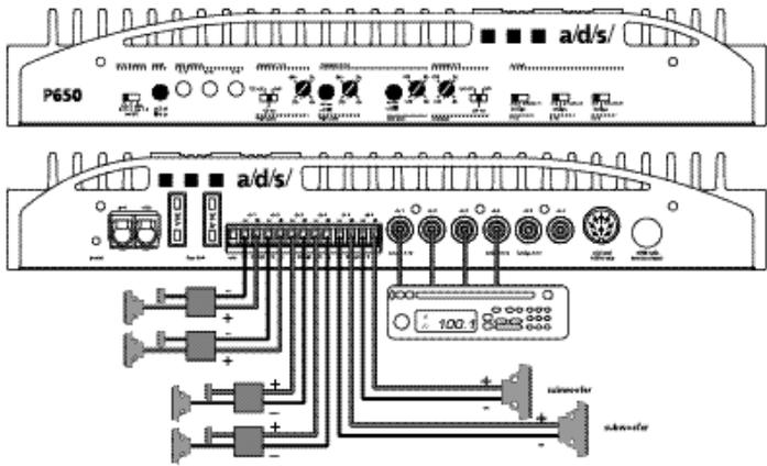
System 2 – P650 used in 6-channel mode. Channels 1/2 are high-passed for front speakers. Channels 3/4 are high-passed for midrange speakers, and channels 5/6 are low-passed for subwoofers.
