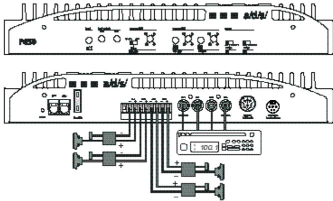
System 2 - P450 used in 2-channel bridged mode with full range speakers.
