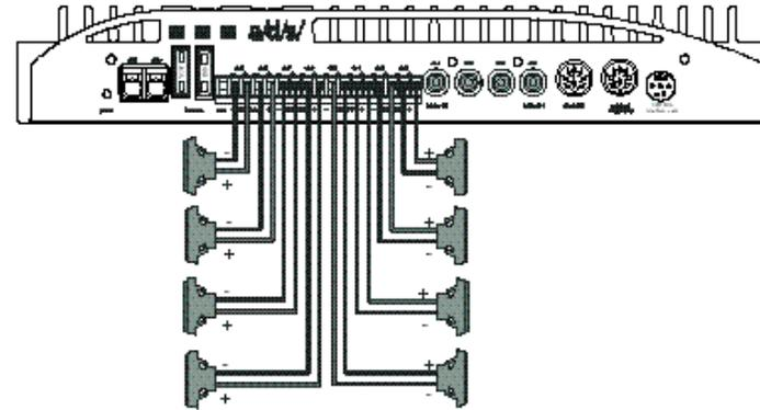
speaker connections for bridged configurations
