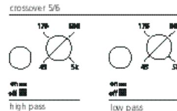
cover control 5/6 (P850) – The crossover section dedicated for channels 5 & 6 are activated by depressing the switch next to the frequency adjustment control. Both high-pass and low-pass crossovers are infinitely adjustable from 45Hz to 5,000Hz. The high-pass and low-pass sections may be combined to create a bandpass filter.
