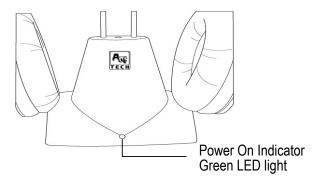
The transmitter will have its power automatically cut off few minutes upon turning off the equipments.
