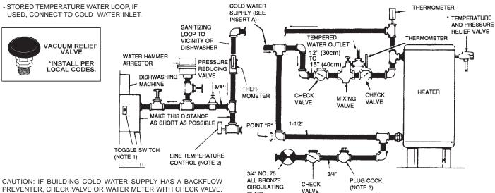
PREVENTER, CHECK VALVE OR WATER METER WITH CHECK VALVE. PROVISIONS FOR THERMAL EXPANSION OF WATER IN THE HOT WATER SYSTEM MUST BE PROVIDED.
