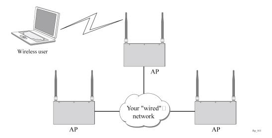
Tropos networks are designed to significantly reduce the wired connectivity requirements of typical 802.11 networks. Only a small number of Tropos Wi-Fi cells, configured as gateways, must be hardwired to your internal network. In fact, for some wireless networks, only one Tropos Wi-Fi gateway may be needed. Additional gateways may be desired provide redundancy and additional bandwidth for larger wireless networks.
