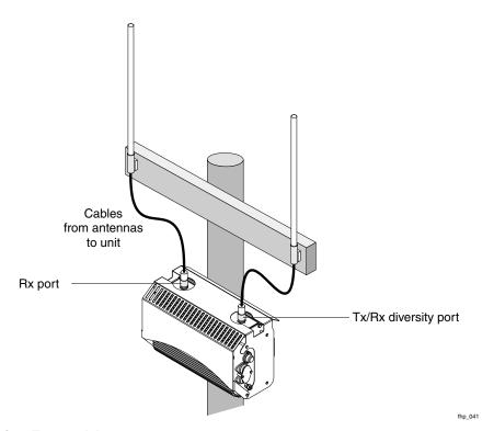
Figure 7 Connecting External Antennas
