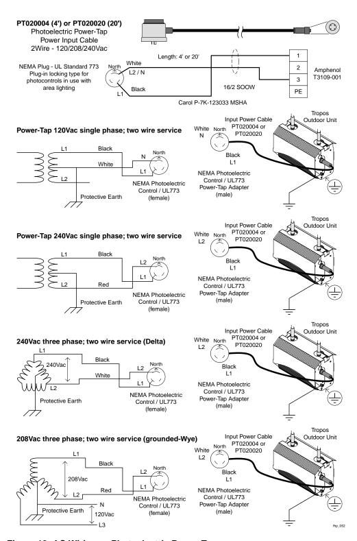
Figure 19 AC Wiring — Photoelectric Power Tap
