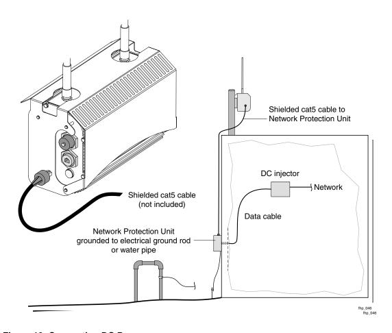
Figure 13 Connecting DC Power
