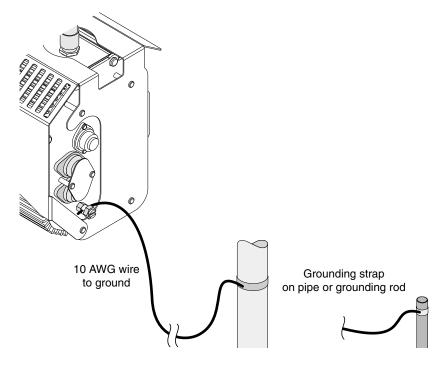
**Figure 10 Ground Post Connection**
