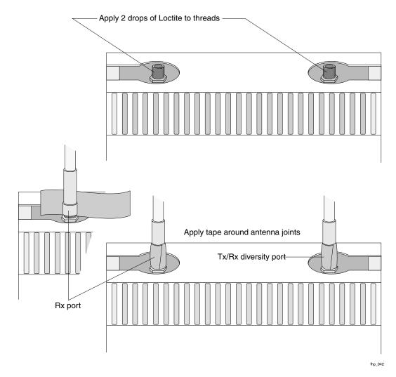
Figure 8 Waterproofing Antenna Connections
