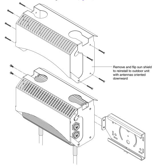
Figure 6 Reattaching sun shield for downward facing antennas
