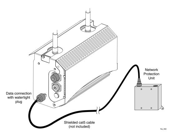
Figure 17 shows how to connect a data cable to the management and LAN ports.
