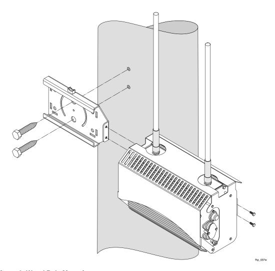
**Figure 3 Wood Pole Mounting**
