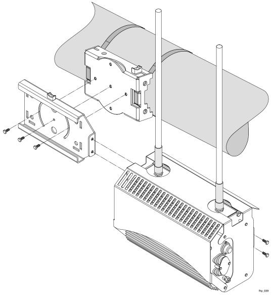
Figure 5 Streetlight Mounting
