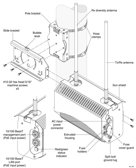
Figure 1 Tropos 5110 Wi-Fi Cell exploded view
