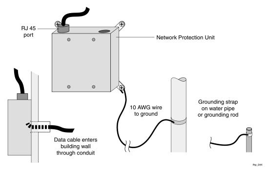
Figure 11 Grounding the Data Protection Device
