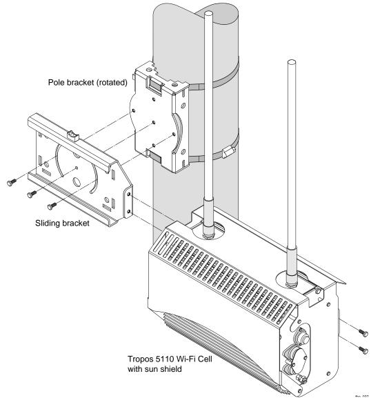
Figure 2 Metal Pole Mounting
