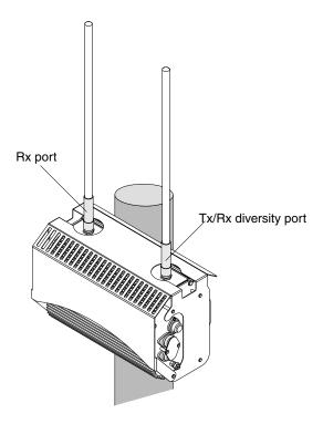
Figure 9 Replacing Tropos 5110 Wi-Fi Cell Antennas
