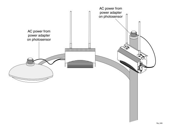
Figure 16 Connecting Streetlight Power
