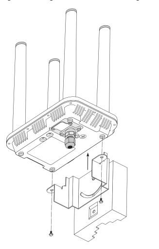
Figure 5 Placing the Router on the Mounting Assembly
