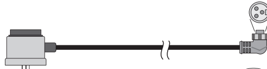
Figure 27 AC Wiring — Photoelectric Power Tap
