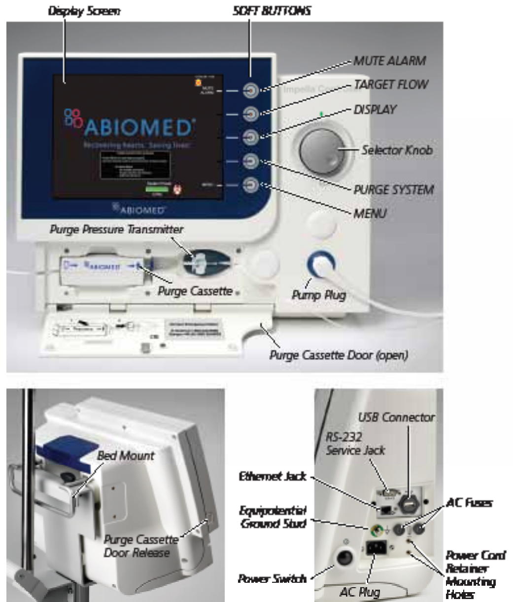
Figure 4.1 Impella® Controller Features – Front and Side Views
