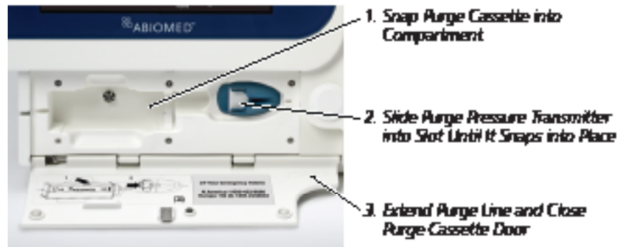
Figure 5.3 Inserting Purge Cassette into Impella® Controller
