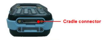
3. Slide the device into the docking station until it clicks into place.
