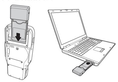
If your laptop does not have a CF or PCMCIA card slot, you need to connect a multi-slot card reader to the laptop, then insert the RF1100 reader into the CF slot as shown.
