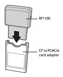
Then insert the RF1100 RFID reader into the PDA or laptop PCMCIA card slot as shown.
