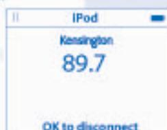
3. Tune the Pico FM Transmitter (A) using the + Up (C) or - Down (D) switches until the desired frequency is displayed. Press and hold for faster tuning. For maximum performance, find a clear frequency with pure static—that is, a frequency with no music or talking, just static.
