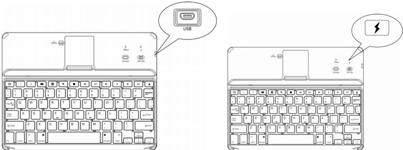
(2)、When you charging, the
