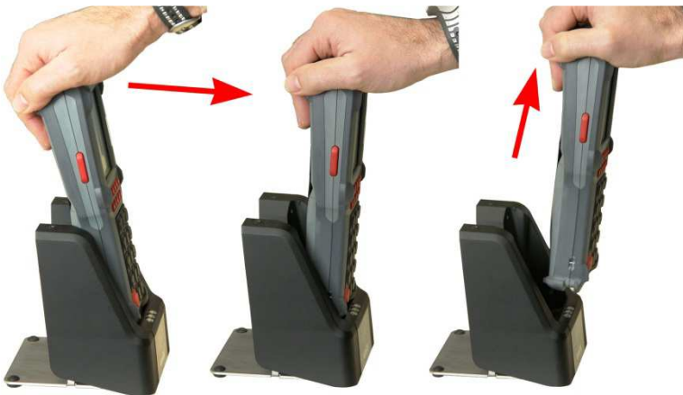
Figure 5: Removing the M260SE from the DS260
