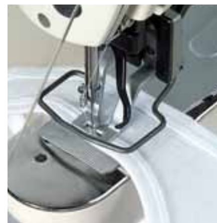
M type (Bartacking shoulder of running shirt)
