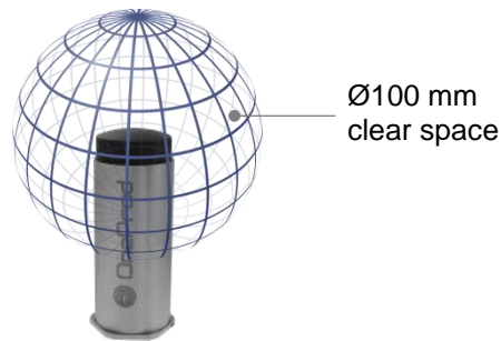
Figure 23 : clear space around the sensor/expander
