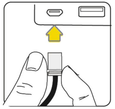
Plug the micro USB connection to the charging port located on the back of the SoundFloe speaker. Connect the power adapter to your wall outlet. Charging will commence automatically.
