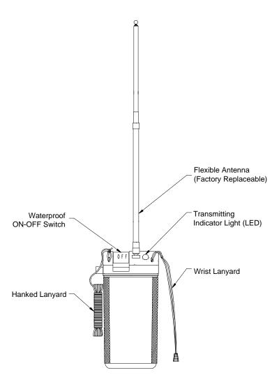
Figure 1: ACR MINI B<sub>300</sub><sup>TM</sup> EPIRB
