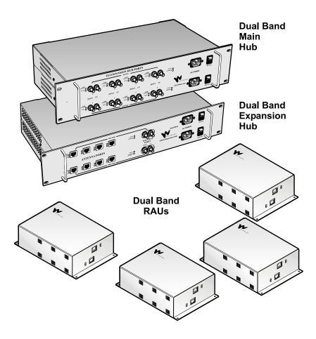
The following sections provide a brief overview of *LGCell* equipment. For a detailed description of the equipment, see *Section 2, LGCell Equipment*.
