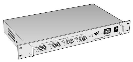
The Main Hub is the LGC*ell*'s central distribution point. It receives downlink cellular or PCS signals from an MBS or a roof-mounted antenna and redistributes them to multiple Expansion Hubs in low-frequency signal format (<200MHz), which can be passed over the MMF and CAT 5 cabling.
