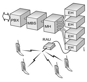
With the LGCell/MBS/PBX solution, employees can use a wireless phone in place of a wireline desk phone to access the PBX while inside the building and use the same phone for wireless communications while outside the building. The MBS private wireless network transmits RF signals indoors, and the macrocellular network takes over outdoors.
