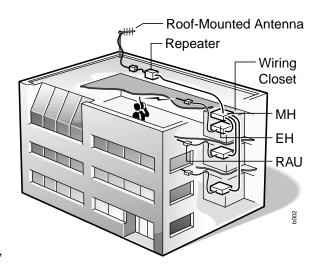
LGCell can be connected to a separate repeater for a power boost or when line of sight is poor.
