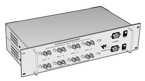
The Main Hub for a Dual Band LGCell system is a pair of Main Hubs, one for each band.
