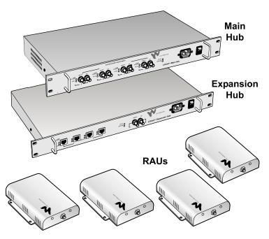
One fully equipped LGC*ell* system consists of the following parts:
