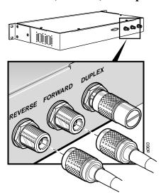
Connect an N-type male RF coaxial cable to the downlink N-type female connector (labeled FORWARD) and an N-type male RF coaxial cable to the uplink N-type female connector (labeled REVERSE) on the Main Hub back panel.
