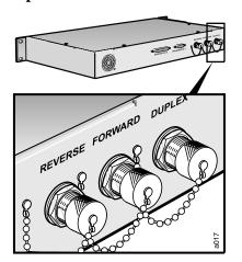
This N-type female connector is typically used to connect the LGC*ell* to a repeater, roof-mounted antenna, or MBS, as shown on the previous page.
