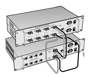
The connections for the Dual Band system are shown here. Make sure you connect the 900 MHz Main Hub to the 900 MHz Expansion Hub and the 1800 MHz hubs together.
