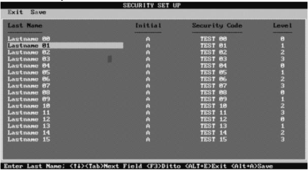
The Security Codes screen enables the system supervisor (highest security, Level 3) to change or add operator names and security codes and assign individual security levels.
