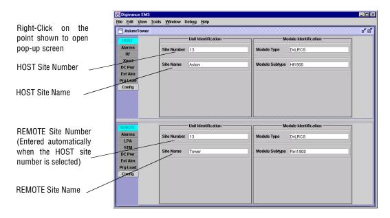
Figure 4-6. HOST and REMOTE Config Displays
