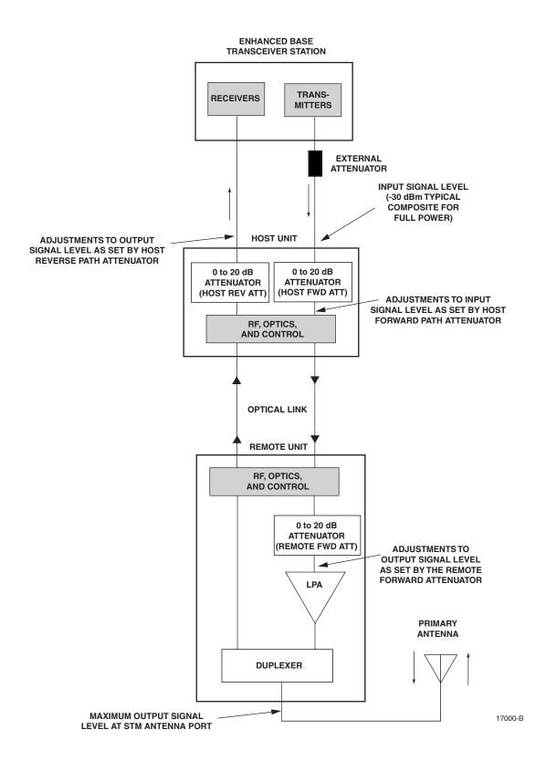
Figure 4-5. Signal Levels, Test Points, and Adjustments
