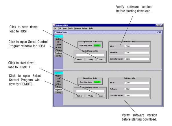
Figure 4-3. HOST and REMOTE Prg Load Displays
