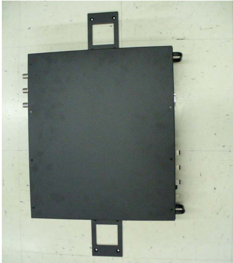
Figure 7-18 Installing Directly to the Wall
