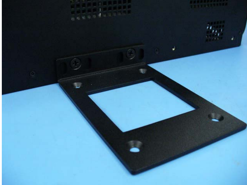
Figure 7-4 Using Hub Rack-Mounting Brackets for Direct Wall Installation
