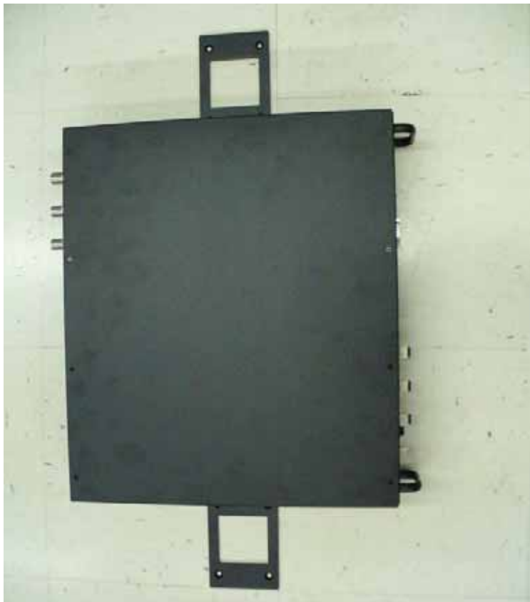
Figure 7-18 Installing Directly to the Wall
