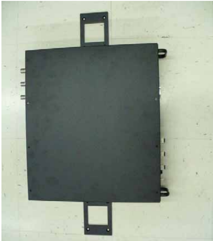
Figure 7-3 Installing Directly to the Wall
