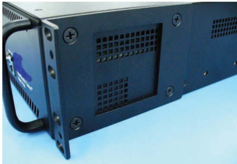
Figure 21. Flush Mounting Bracket Detail
