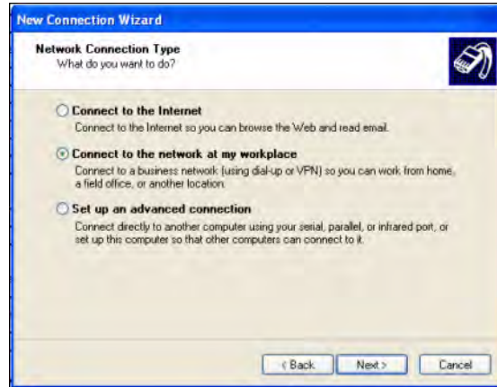
Figure 7-43 New Connection Wizard - Network Connection Type Window
