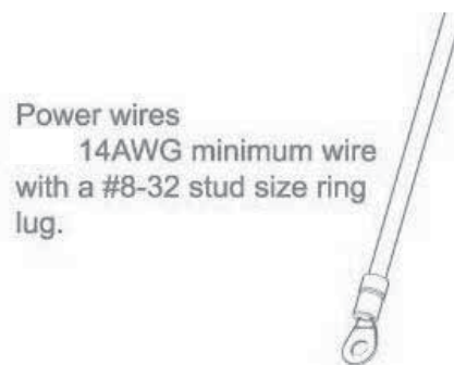
Figure 7-12 Power Wires and Studs
