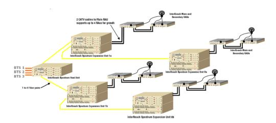
You add bands by inserting DART cards and CATV jumper between the Main and new Secondary RAUs, as shown below. 1 to 16 cascaded Expansion Units support up to 128 RAU locations.
