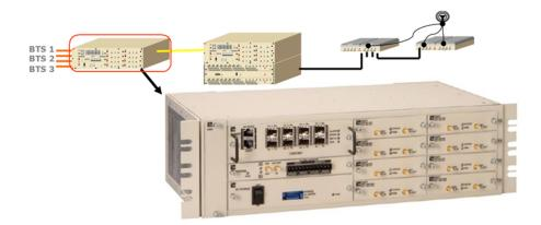
The Host Unit is installed into a 19-inch, rack-mounted chassis, that is 9-inches deep and can hold up to three Host Units. Each Host Unit can have up to eight hot swappable plug in cards. Host Unit components are as follows:
