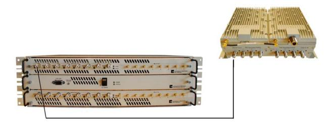
**5** Connect F connector CATV cable from IFEU REV Module Port IF IN to MRAU REV IF OUT F connector.
