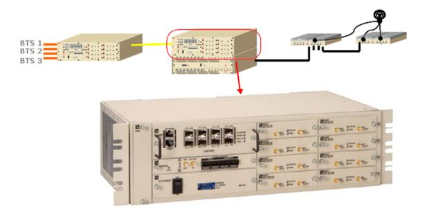
The DART Remote Unit (DRU) is installed into a 19-inch, rack-mounted chassis, that is 9-inches deep and can have up to eight hot swappable plug in cards. DRU components are as follows:
