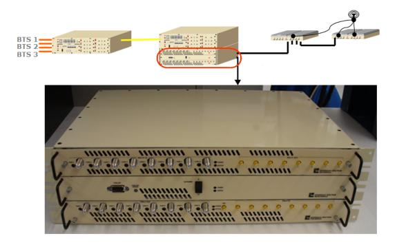
The IF Expansion Unit (IFEU) is installed into a 19-inch, rack-mounted chassis, that is 15-inches deep with three plug-in cards. IFEU components are as follows:
