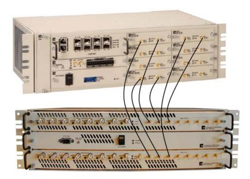
**4** Connect F connector CATV cable from IFEU FWD Module Port IF OUT to MRAU FWD IF IN F connector.
