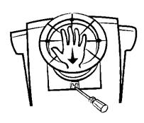
To remove the assembly base, press down the lock with a screwdriver and remove the base in the direction of the arrow.
