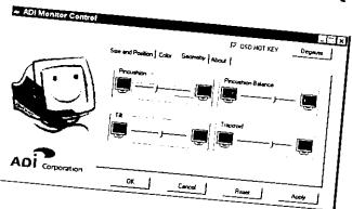
Click on any one of the parameters with your mouse, and use left/right arrow keys on your keyboard to adjust. You may also drag the cursor of a parameter toward left/right for adjustment.
