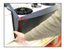
18. Remove the cap from the cooling barrel.
