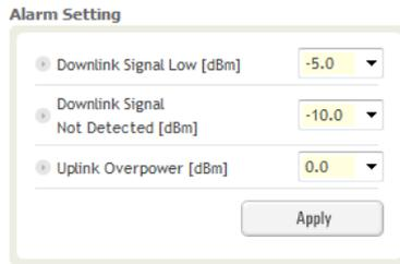
**Figure 8-48 Alarm Threshold Setting (Control – RFU)**
