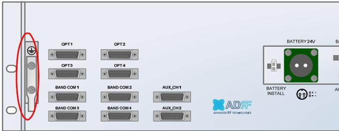
Figure 6-5 Ground Cable Connection (HE rear side)
