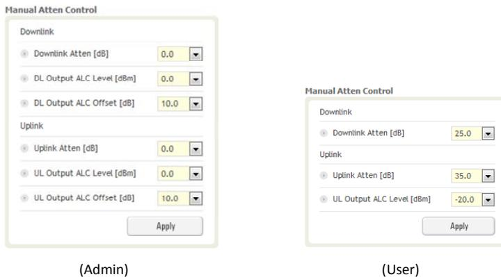
**Figure 8-47 Manual Attenuator Control Setting (Control – RFU)**
