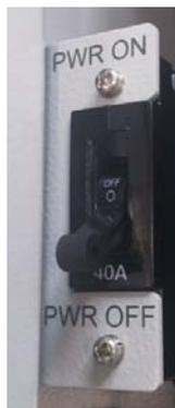
**Figure 3-29 HPR AC Switch**
