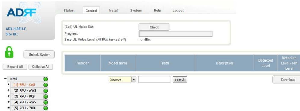
**Figure 8-46 UL Noise Detection - PCS band**
