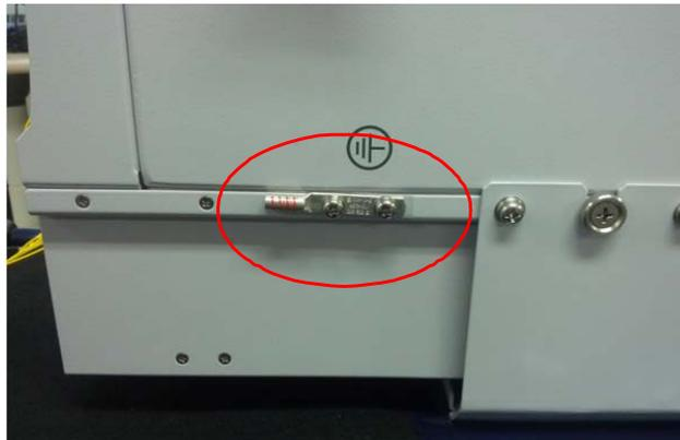
Figure 6-6 Ground Cable Connection (HPR dual side)
